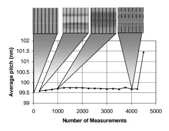
Fig. 2 E-beam induced degradation of the pitch standard and change in measurement result
