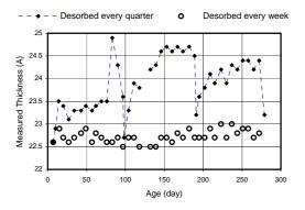
Fig. 9 Film thickness variation over time; quarterly desorption performed on 98<sup>th</sup>, 191<sup>st</sup>, and 271<sup>st</sup> day.
