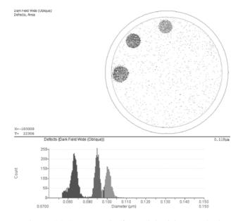
Fig. 10 SSIS scan result of a particle sizing standard
