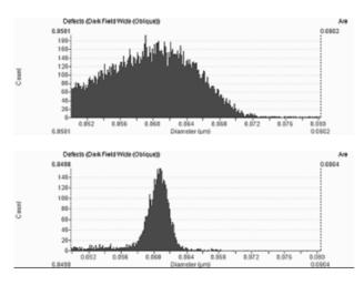
Fig. 11 SSIS histograms of original (top) and DMAselected (bottom) 60 nm PSL sphere depositions
