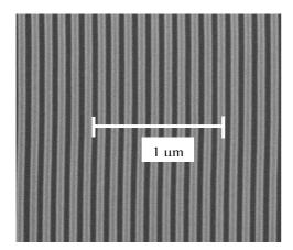
Fig 1. CD-SEM image of a 100 nm pitch standard
