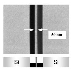
Fig. 3 CD-SEM image and structure illustration of a 50 nm CD standard
