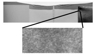
Fig. 4 TEM images showing the cross section of a 25nm polysilicon line and the atomic lattice of the crystalline Si subsrate.
