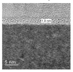
Fig. 7 TEM cross section image of a  $SiO_2$  film thickness standard of about 1.9 nm physical thickness; a poly-Si cap layer was deposited on the sample to obtain a better defined  $SiO_2$  surface for the TEM image.
